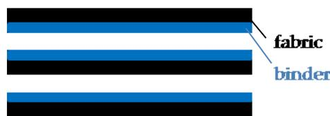
Fig. 1: Lay-up and binder orientation
