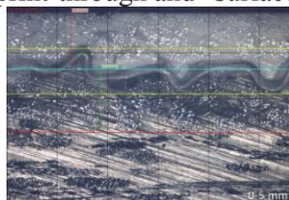
Figure 3: Typical cross-section of a composite with the Baltex separator fabric showing wrinkling of the separator layer substrate (the continuous line from left to right) and the larger separator layer fibres in both the gel coat (above) and the laminate (below).
