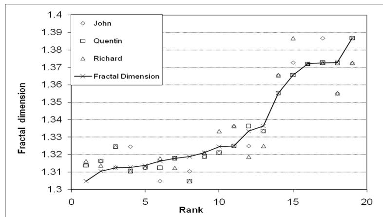
Figure 5: Correlation of the fractal dimension and human assessment of gel coat quality
