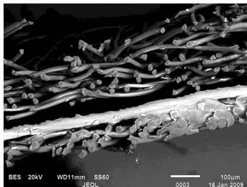
Figure 1: A section through a typical trilaminate separator layer.
