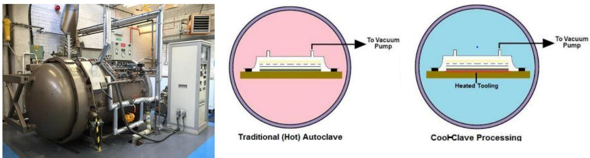
Figure 1: The Plymouth autoclave (left), schematic of conventional autoclave (centre), cool-clave (right).
