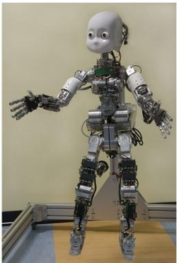
The iCub is an open source cognitive humanoid robot platform. It has 53 motors that move the head, arms & hands, waist, and legs. It can see and hear, it has the sense of proprioception (body configuration) and movement (using accelerometers and gyroscopes).
