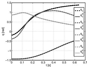
Figure 3: Joint angle trajectories corresponding to a typical reaching movement (data captured from an adult). Solid lines,  $q$ , correspond to captured data. Dashed lines,  $q_d$ , correspond to the trajectories performed when the feedforward controller perfectly inverts the dynamics of the artificial arm ( $\hat{M} = M$ ,  $\hat{C} = C$ ,  $\hat{G} = G$ ). Clearly, resulting trajectories corresponded to the desired one ( $q \equiv q_d$ ).
