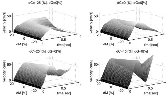
Figure 5: Four examples ( $dC = -25\%$ ,  $dC = 25\%$ ,  $dC = 50\%$  and correct estimate  $dC = 0\%$ ) of Coriolis forces miscalculation in a pure feedforward controller as a function of changing estimates of inertial torques. Remarkably, relevant overestimates of the Coriolis component produce double peak velocity profiles which were not present in case of inaccurate gravitational and inertial components.
