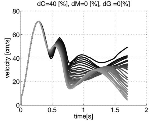
Figure 6: The effect of delayed feedback on hand trajectory formation. Shown are velocity profiles when the controller approximated dynamics did not match the Coriolis arm dynamics. ( $\hat{C}$  overestimates  $C$  of a 40%). After 300 ms position feedback became available. The various profiles show the effect of different feedback gains: the darker the line the smaller the overall feedback gain  $k = k_p + k_v$  is (see footnote 1 at page 2 for the definitions of  $k_p$  and  $k_v$ ).
