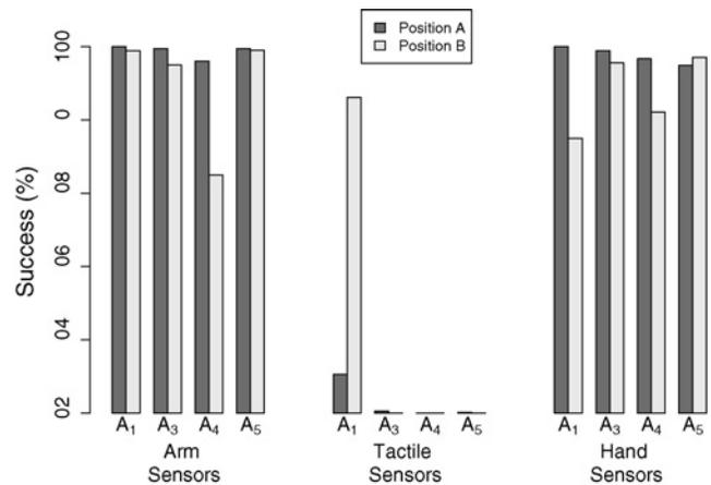
Fig. 5. Graphs showing, for agents  $A_1$ ,  $A_3$ ,  $A_4$ , and  $A_5$ , the results of substitution tests concerning the readings of arm proprioceptive sensors, tactile sensors, and hand proprioceptive sensors for position A (see black columns) and for position B (see gray columns).
